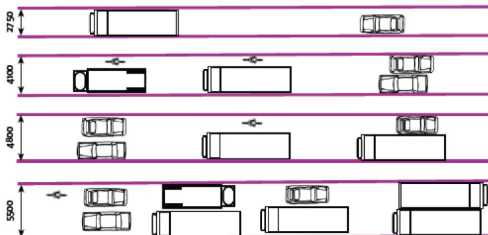
Figure 7.1 illustrates what various carriageway widths can accommodate. They are not necessarily recommendations.
